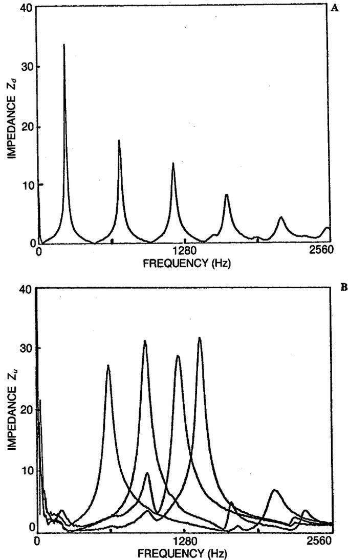
Fig. 2. A. Impedance  $Z_d$  looking downstream from the reed into a clarinet fingered to give  $C_4$ . B. Impedance  $Z_u$  looking upstream into the player's windway for several vowel-like configurations of the mouth and throat.
